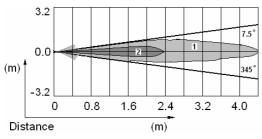
Curve 1: flat surface 100 mm x 100 mm Curve 2: flat surface 50 mm x 50 mm
